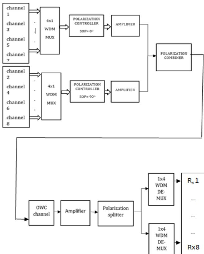
**Fig.2 Block diagram of Is-OWC WDM system with polarization-interleaving**
