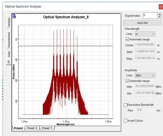
Fig: 3 transmitted signal power spectrum of OFDM
