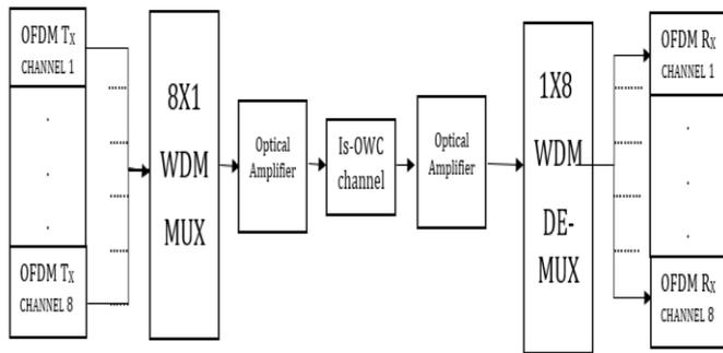
**Fig. 1 Block diagram of an Is- OWC OFDM WDM SYSTEM**
