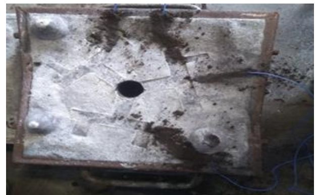
Figure2. Mold with thermosensors probe
