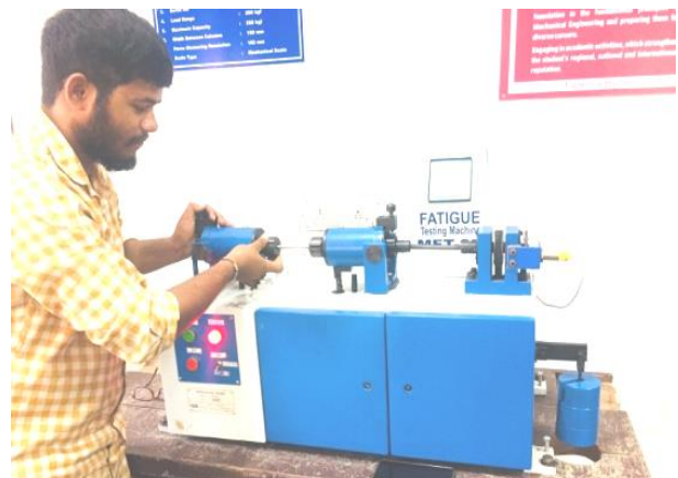
Fig- 3 (b): Mounting of specimen on the FTM
