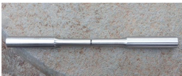
Fig-2(b): Notched Specimen
