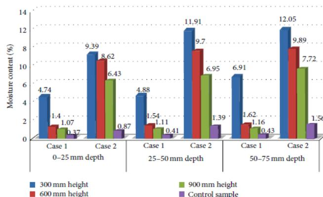
Fig. 4.1 Comparisons of Moisture Content at Different Heights for Differing Depth of Walls
