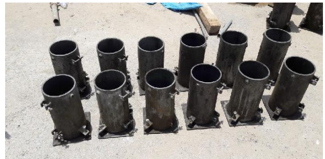
Figure: casts of cylinders for compressive test
