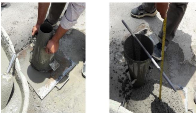
Figure(a) Removing Cone (b) Height Measurement
