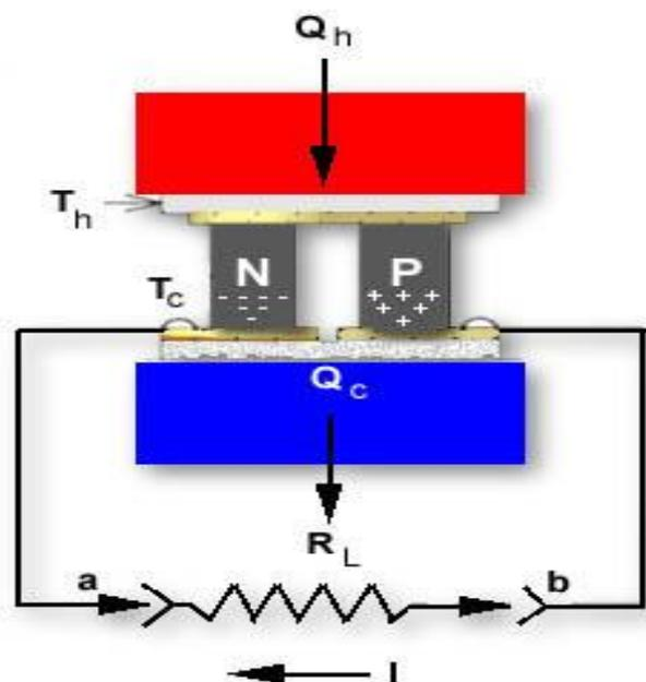
**Figure 6 Electricity Generation With One Thermoelectric Power Module [15]**
