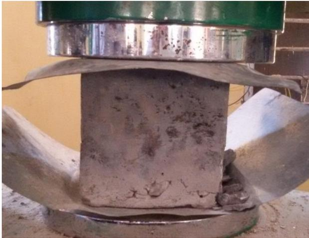
**Fig 4 - compression Testing of Concrete cube specimen**
