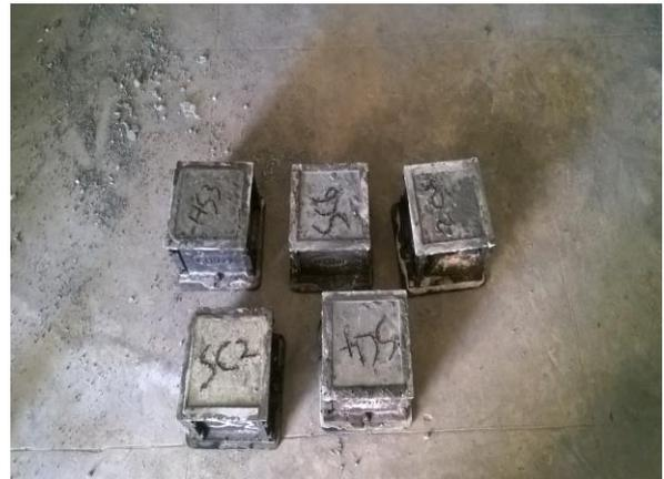
**Fig 3 – Casting of concrete specimens**
