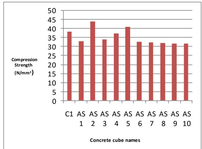
**Chart -1:** Compression strength (N/mm<sup>2</sup>) values for all concrete cube specimens
