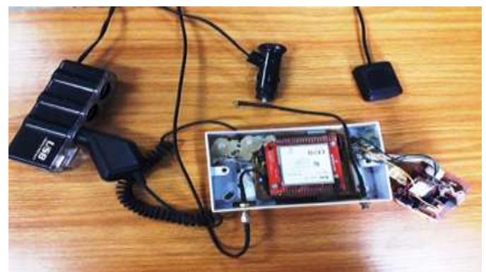
Fig -3: Internal Circuitry of Implemented Over-speed Reporter.
