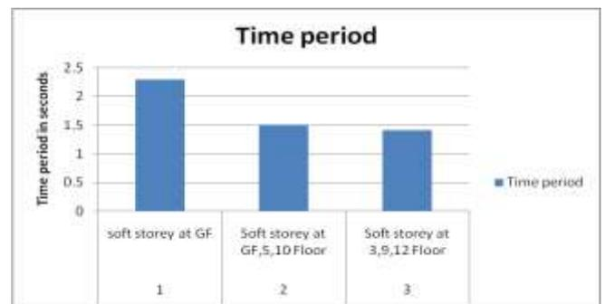
**Fig 8: Graph of time period of models with shear wall for seismic zone III & V.**
