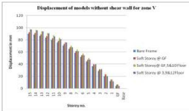
**Fig 5: Graph of displacement of model without shear wall for Zone V in x direction.**
