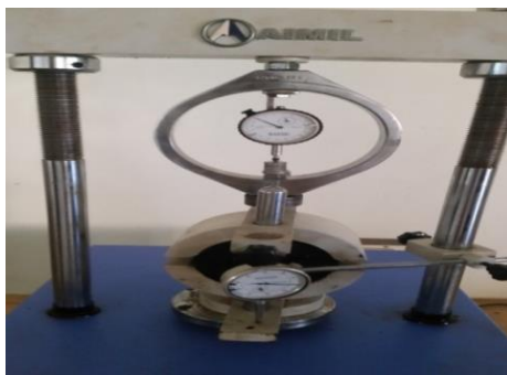
Fig 4: Marshall stability test
