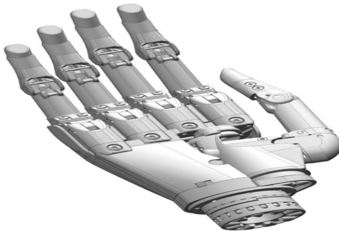
Fig. 2 An illustration of the Limb hand as an example of a modern prosthetic hand demonstrating the modular assembly and aesthetic appearance of currently available prostheses
