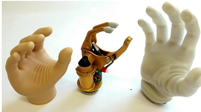
Figure 3 Examples of Otto bock prosthetic hands and cosmetics (from left to right): small System Inner Hand, small MyoHand VariPlus Speed, and medium Michelangelo hand.
