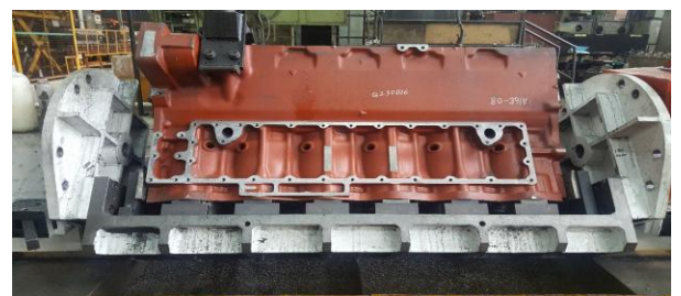
Fig -14: Engine block mounted on Indexing Fixture for Reworking
