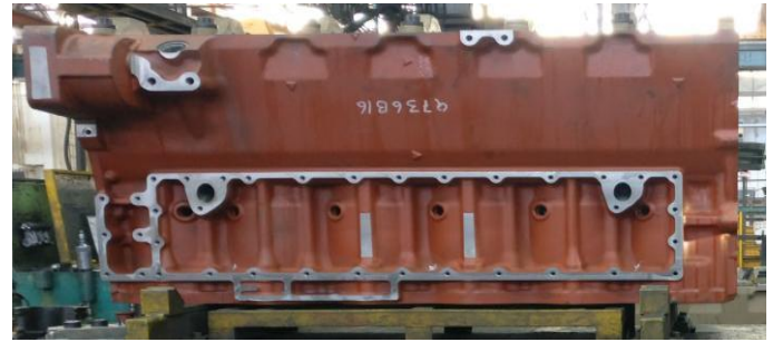
Fig -1: Engine block on which reworking is done
