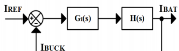
Fig. 6. Control of Buck Converter.
