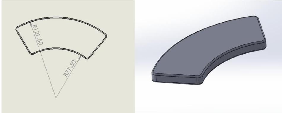
**Figure- 2:** (a)Initial sketch of TEG unit, (b)Final model of TEG unit
