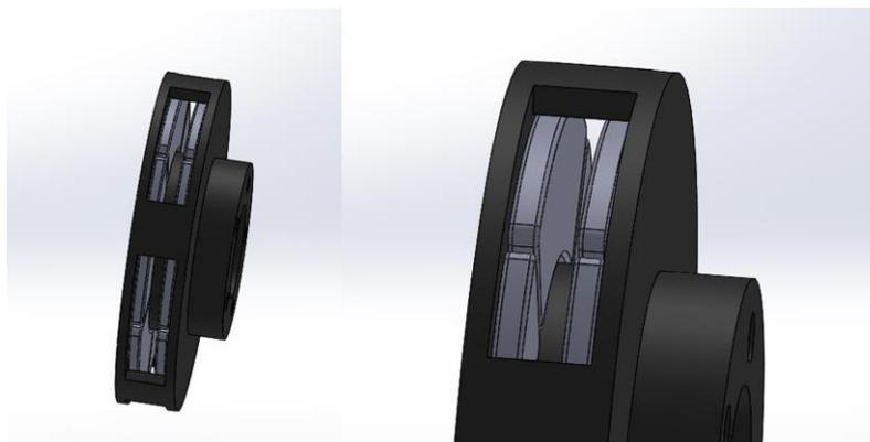
Figure- 7: Installation of TEGs on the inner sides of the disc
