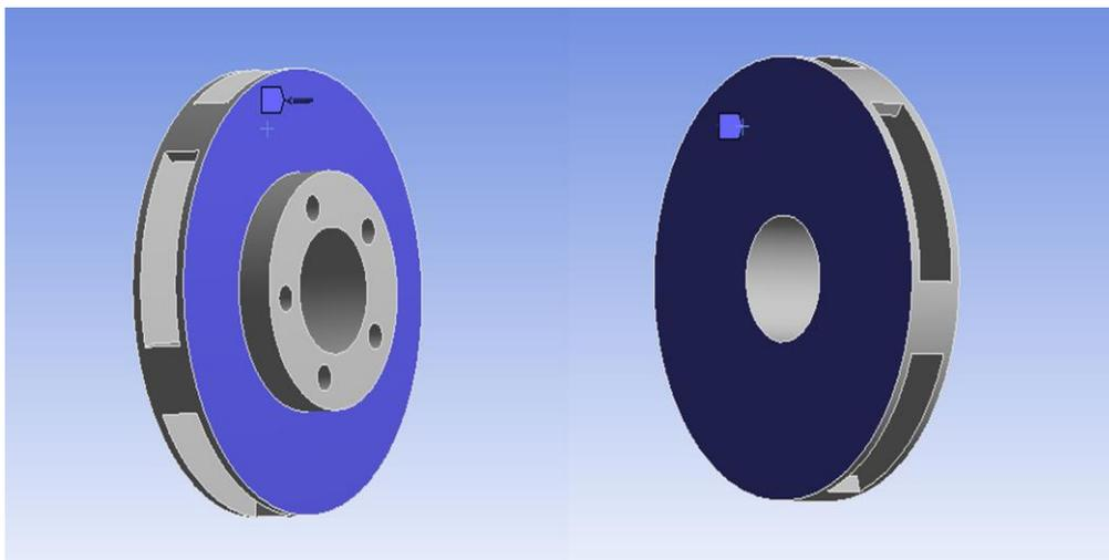
**Figure- 4:** (a)Heat flow on the first surface, (b)Heat flow on the second surface
