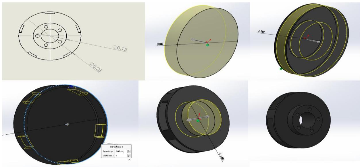
**Figure-1:** (a) Initial sketch of disc, (b) Outer circle extrusion, (c) Inner circle extrude cut, (d) Support Ribs, (e) Hub support and (f) Disc final model
