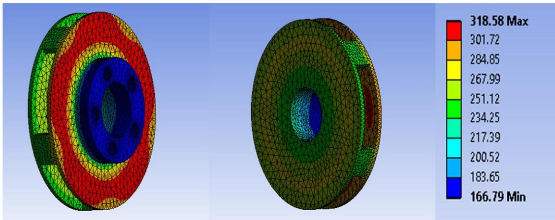
Figure- 6: Temperatures of different zones in a disc
