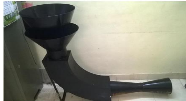
Fig -8: Full assembly of Ducted Wind Turbine
