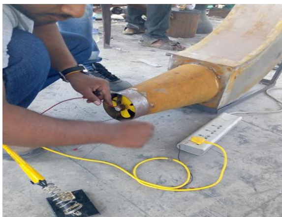
Fig -6: Soldering of motor wire connection
