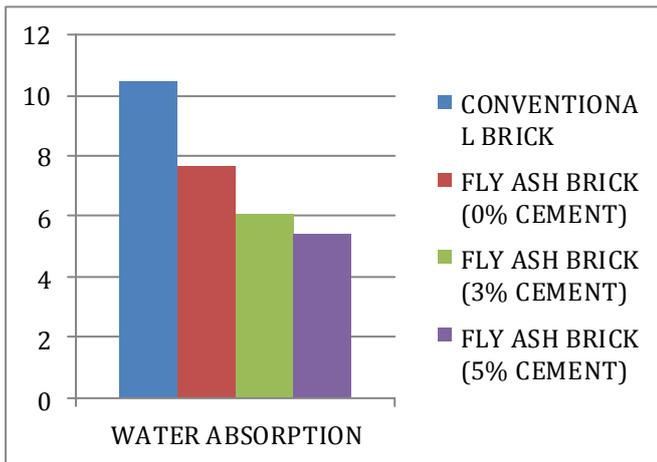
Figure 3 Water Absorption Test Results
