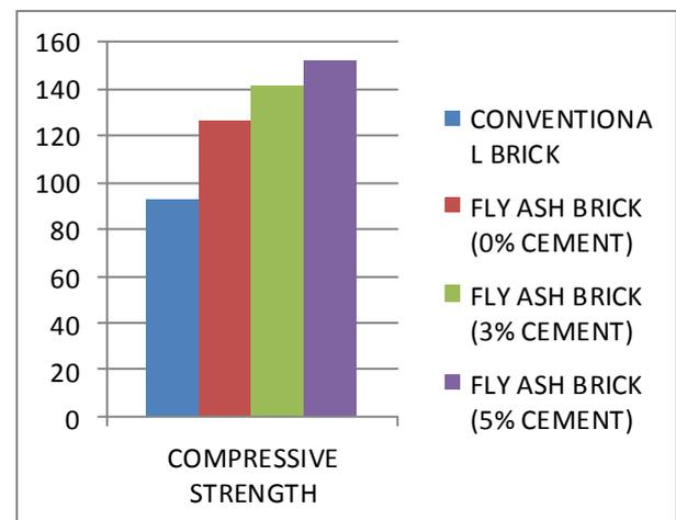
Figure 2 Compressive strength Test Results
