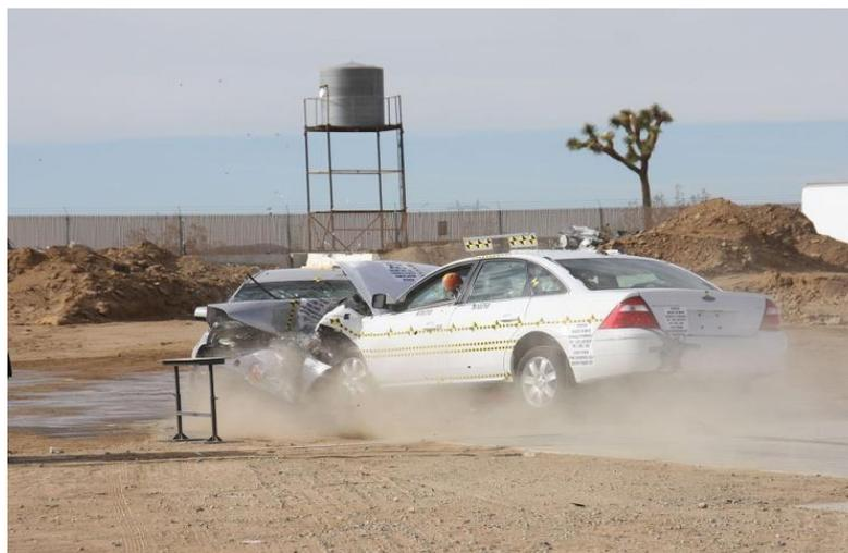
Figure 3: NHTSA research crash test carried on two Ford 500.
