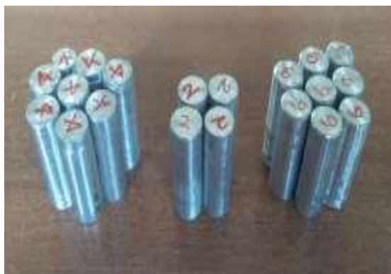
Fig 2. Specimen Pin For Wear Test.
