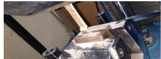
Fig. 2.2. Fracture on peel test diagram
