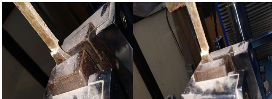
Fig. 1.2. Fracture on lap shear test diagram
