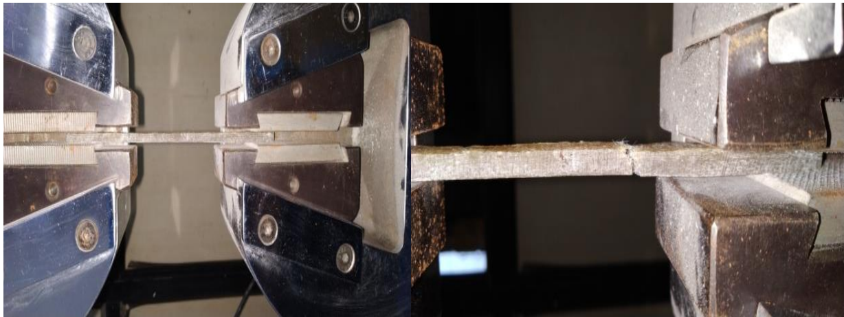
Fig. 3.2. Fracture on tensile test diagram
