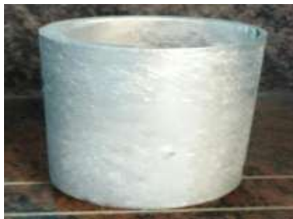
Fig-2.2 Mold formed after centrifugal casting
