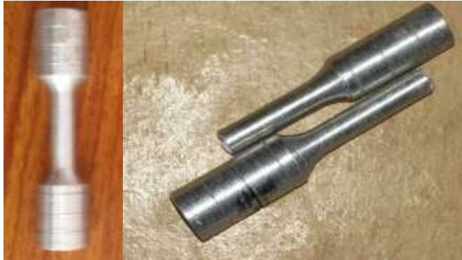
Fig-3.3 Tensile specimen before and after breaking
