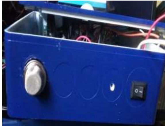
Fig 3.9: MQ4 Gas sensor connected to the packaging box.
