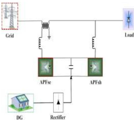
**Fig -1:** Basic structure of UPQC with distributed generation
