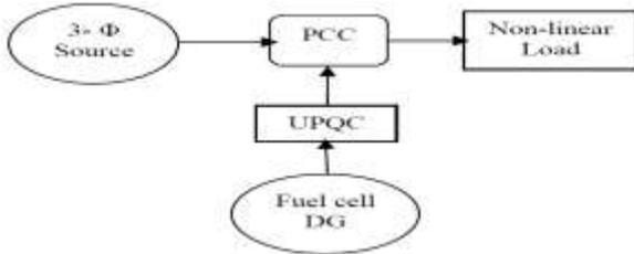
Fig -2: Integration of UPQC between Fuel cell and PCC
