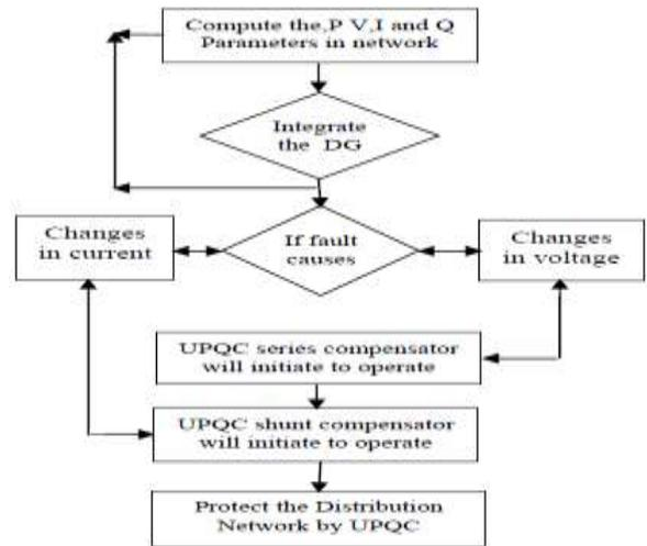
Fig -4: Flow chart for the analysis of compensation of reactive power
