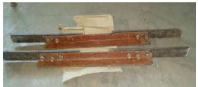
Fig. 1: Test Specimen of Tension member
