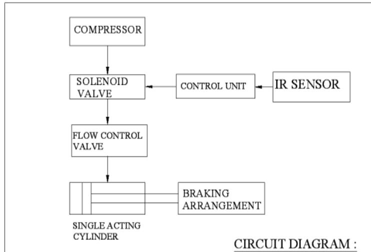
**Fig. 4** Flow Diagram
