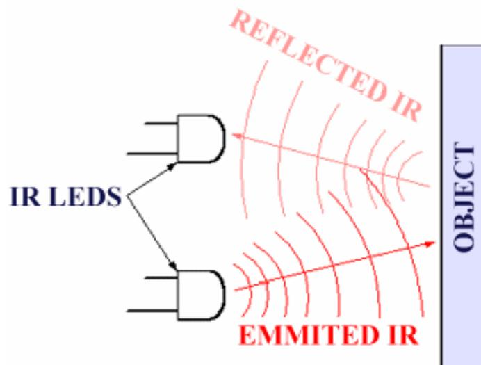
Fig.3 Working of IR Sensor
