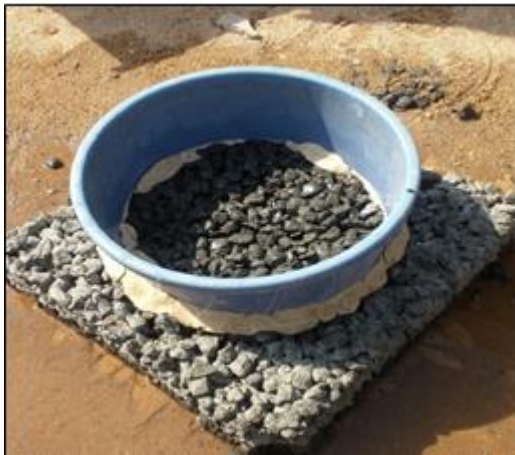
Fig -1: Infiltration test
