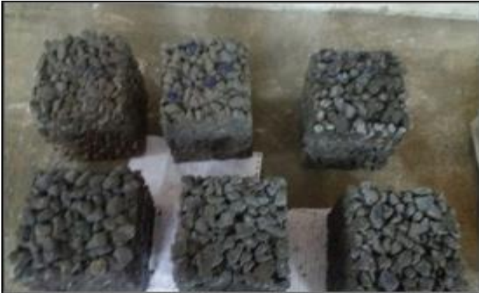
Fig-2: Pervious Concrete Cubes
