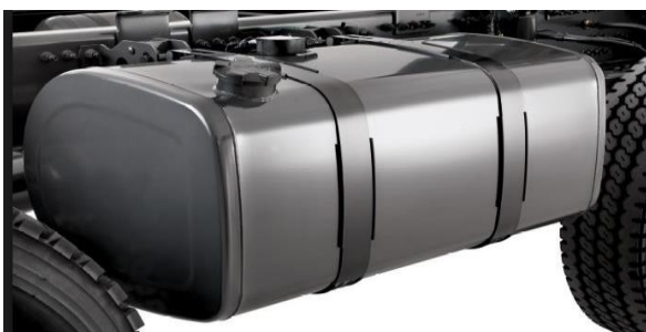
Fig -1: fuel tank and mounting bracket of truck
