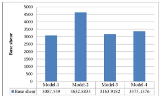
Fig 4.11: Base Shear by RSA along X-Direction
