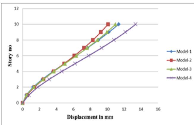
Fig 4.8: Story Displacement by RSA along Y- Direction
