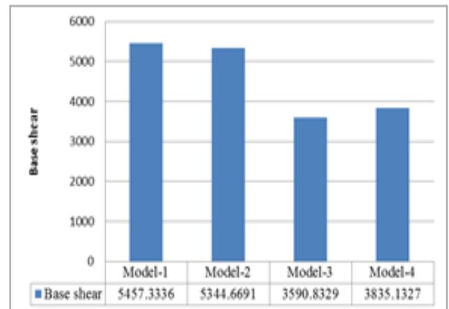
Fig 4.5: Base Shear by ESA along X-Direction
