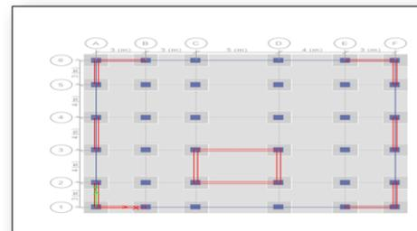
Fig 3-Plan view of flat slab with shear wall
