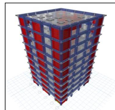
Fig 4- 3D View of flat slab with shear wall
