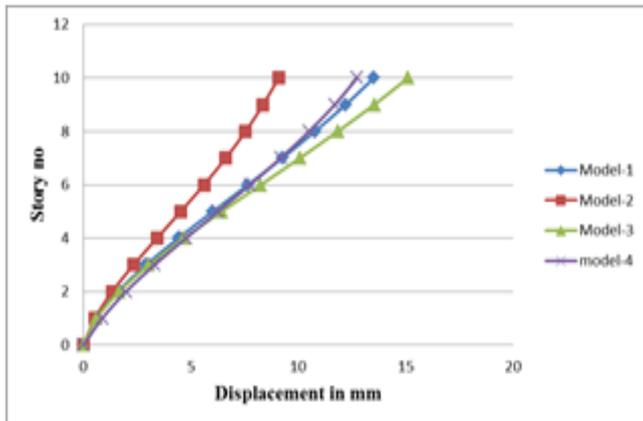
Fig 4.7: Story Displacement by RSA along X- Direction
