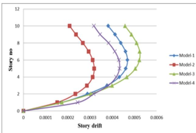
Fig 4.9: Story Drift by RSA along X-Direction
