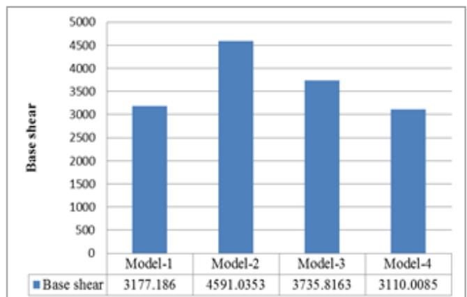
Fig 4.12: Base Shear by RSA along Y-Direction
