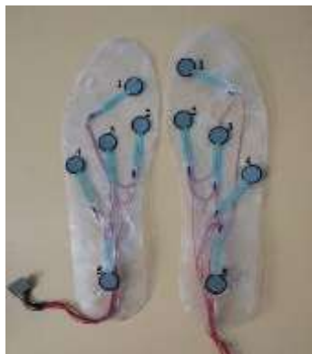
Fig -2: FSR position at Hallux (1), Medial forefoot (2), Central forefoot (3), Lateral forefoot (4), and Heel (5).
