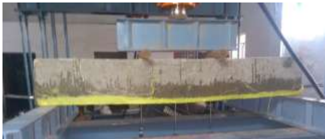
Fig 6:- Deflected shape of Post Tensioned Beam
