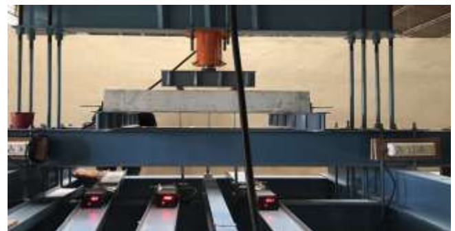
Fig 5:- Test setup for Post Tensioned Beam
