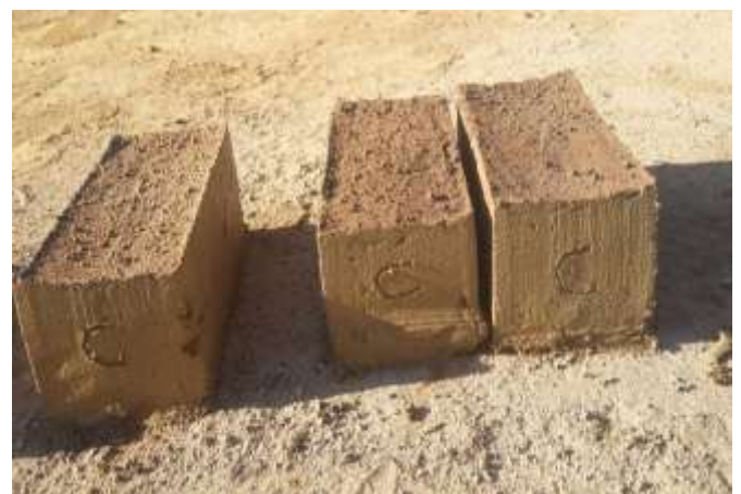
Fig-6: Geopolymer Bricks with Material Ratio 80:20
