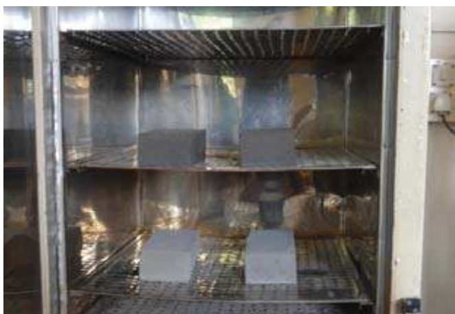
Fig-4: Dry Hot Oven Curing
