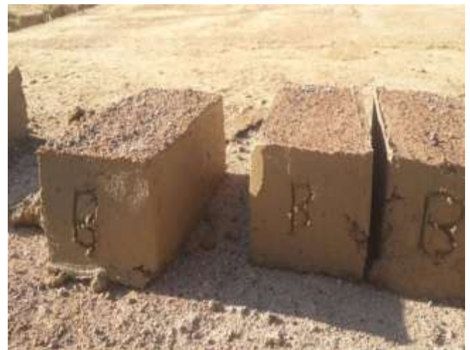
Fig-5: Geopolymer Bricks with Material Ratio 70:30
