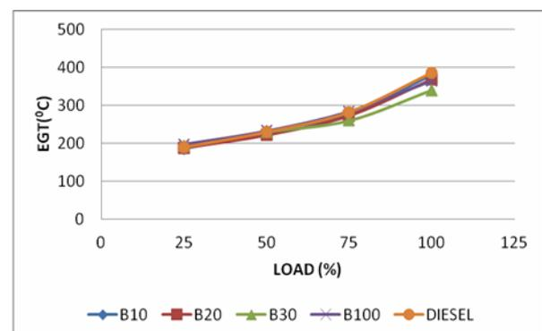
Fig -5: Load v/s Exhaust gas temperature
