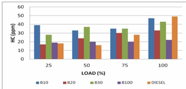
Fig -6: Load v/s Hydrocarbon
