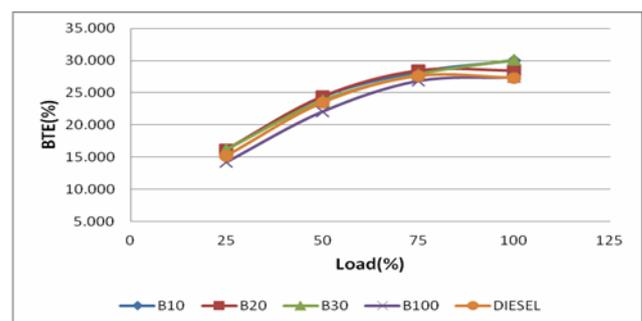
Fig -4: Variation of brake thermal efficiency with load
