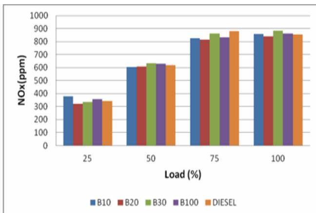
Fig -7: Load v/s Oxides of Nitrogen
