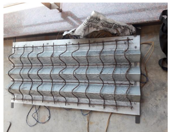
Fig-1: Ferrocement slab with single layer wire mesh
