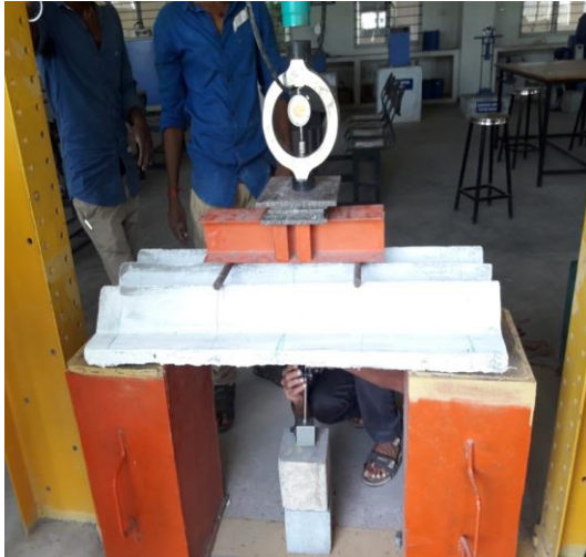
The geometry of the panel is flat shape as shown with dimensions 1000 mm x 400 mm x 30mm
