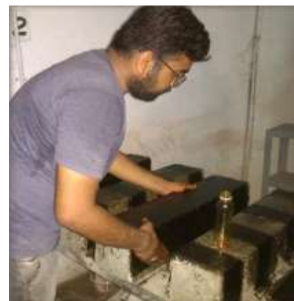
Fig-5: Surface Preparation and Applying Basalt fiber on Beam.
