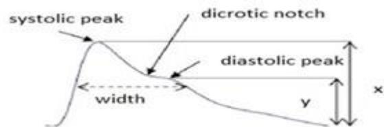
Fig 1: Typical PPG signal
