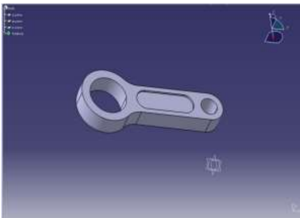
Fig 3: Reversed cad developed design of connecting rod
