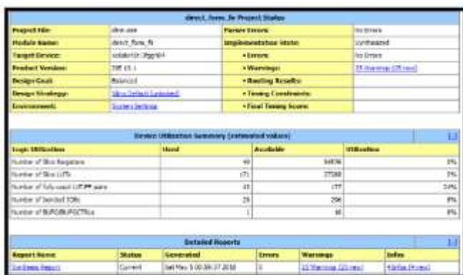
Figure 8: Synthesis Output of Direct Form Transpose of Spartan 6.
