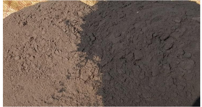
Fig -4: Cow dung and sugar cane bagasse ash mixture
