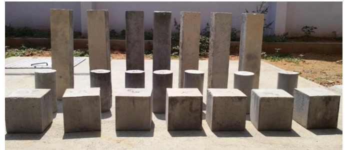
Fig -5: Demoulded and cured specimens at 28 days
