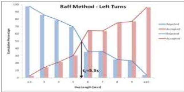
Figure 3.2: Graph showing gap length by Raff method
