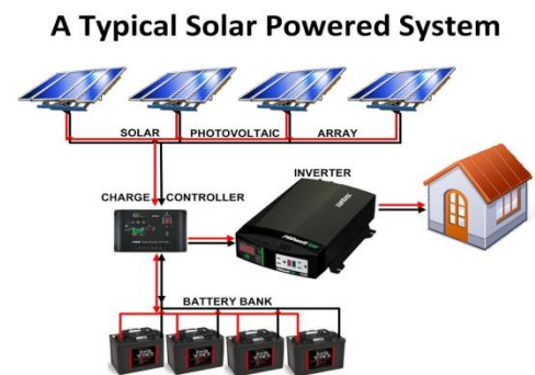
Fig 1: Typical Solar Power System
