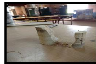
Fig 2: UCC specimen after failure.
