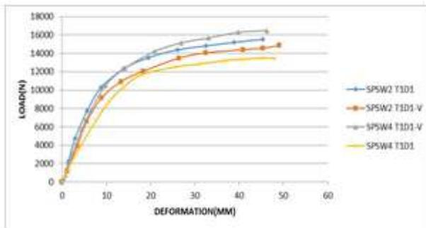
Fig 5: Load-Displacement curveor holes with different patterns of T1 thickness 75mm dia
