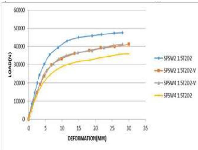
Fig 11: Load-Deformation curves for holes with different patterns of T2 thickness 100mm dia
