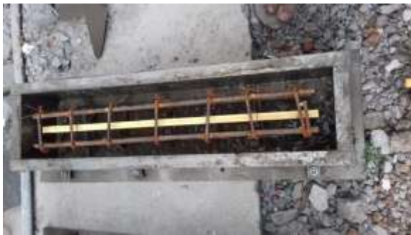
Fig -4: Casting of I-section GFRP beam
