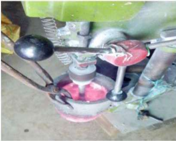
Figure.11 Stirring of red mud particles with molten Al6061
