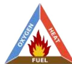
**Fig -2:** The Fire/Combustion Triangle
