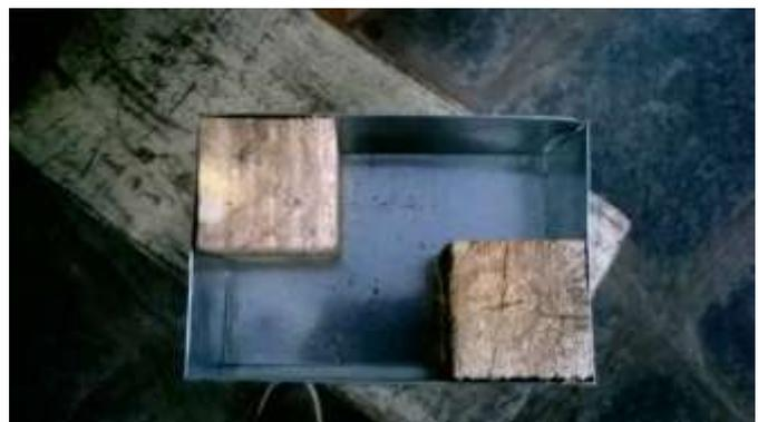
**Figure -2:** Fabricated Z-shape mold
