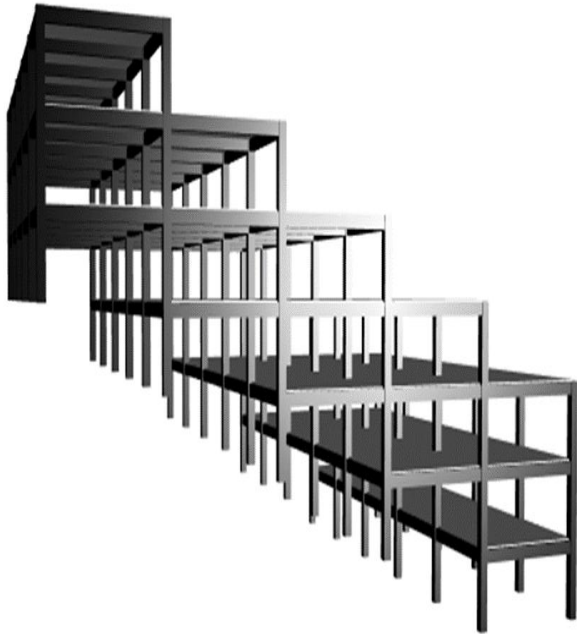
Figure 9: Rendered view of 5 bays step-back setback building.
