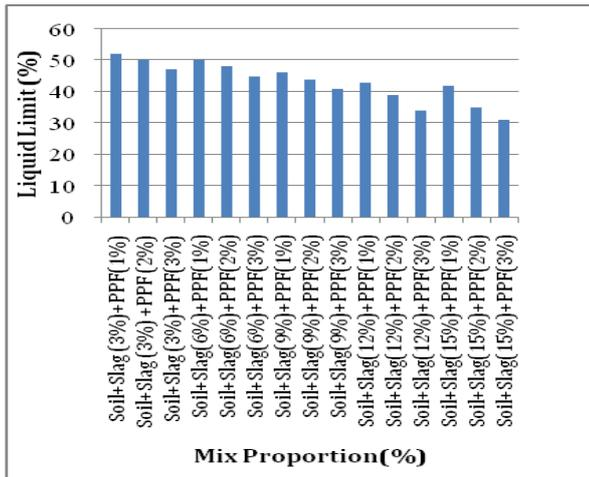
**Chart-2:** Variation of Liquid Limit with addition of different proportion of Steel Slag and Polypropylene Fibers
