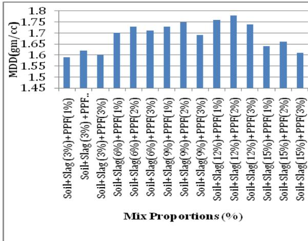
**Chart-3:** Variation of Maximum Dry Density with addition of different proportion of Steel Slag and Polypropylene Fibers
