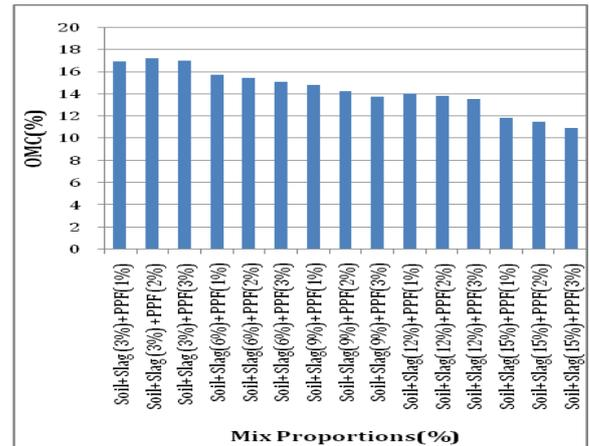
**Chart-4:** Variation of Optimum Moisture Content with addition of different proportion of Steel Slag and Polypropylene Fibers
