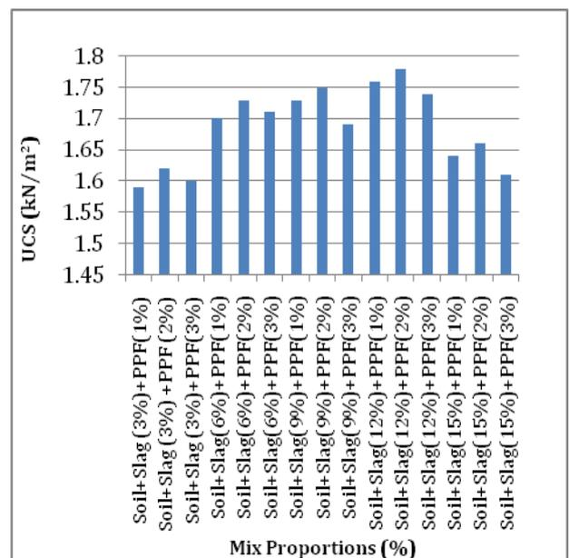
**Chart-5:** Variation of UCS with addition of different proportion of Steel Slag and Polypropylene Fibers
