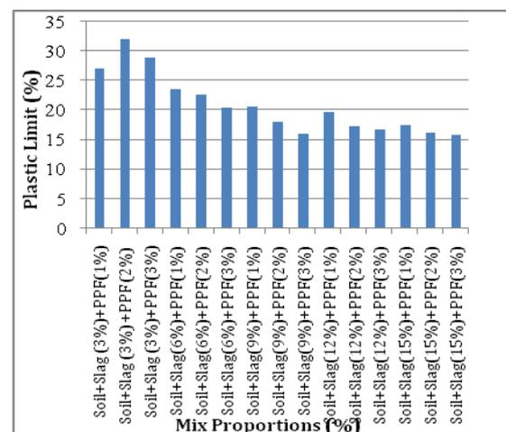
Chart-1: Variation of plastic limit with different proportion of steel slag and Polypropylene fibers
