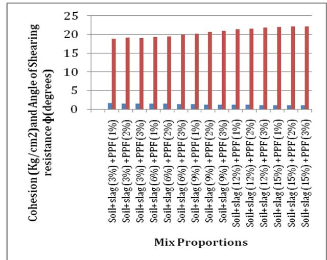
**Chart-8:** Variation of Cohesion and Angle of shearing resistance with addition of different proportion of Steel Slag and Polypropylene Fibers
