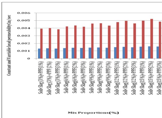
**Chart-7:** Variation of Permeability with addition of different proportion of Steel Slag and Polypropylene Fibers
