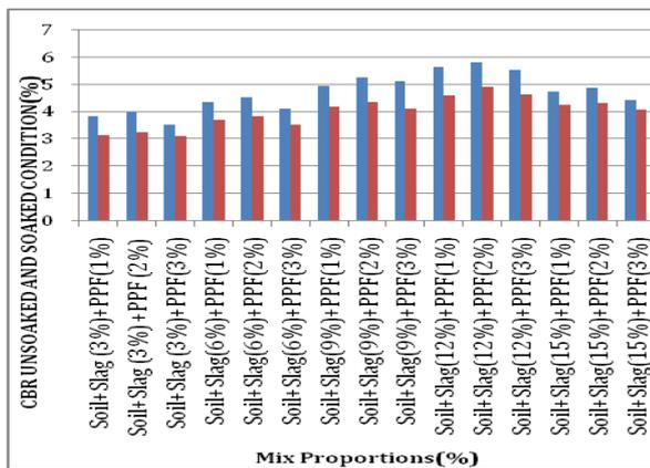
**Chart-6:** Variation of CBR with addition of different proportion of Steel Slag and Polypropylene Fiber.
