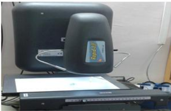
Fig. 7 Rapid-I Vision Inspection System
