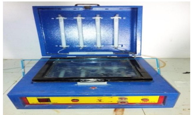
Fig.5 Ultraviolet Light exposure unit
