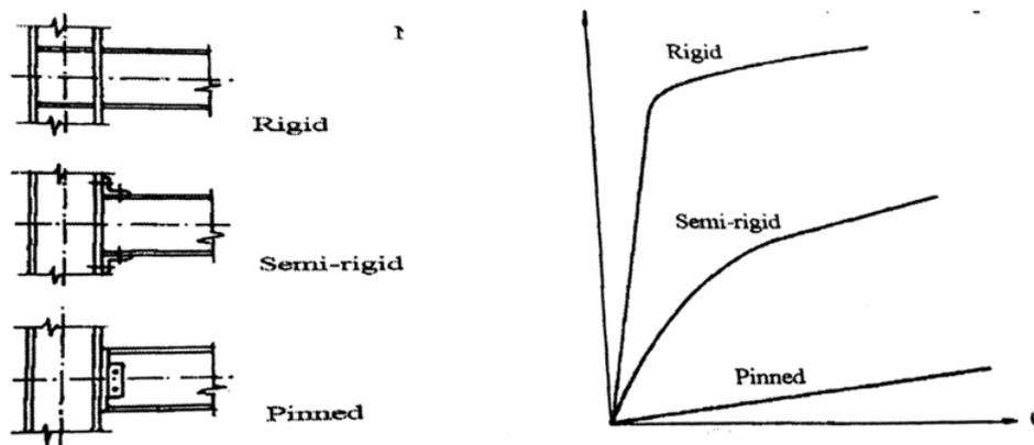
Fig. 1 : Types of beam-to-column connections
