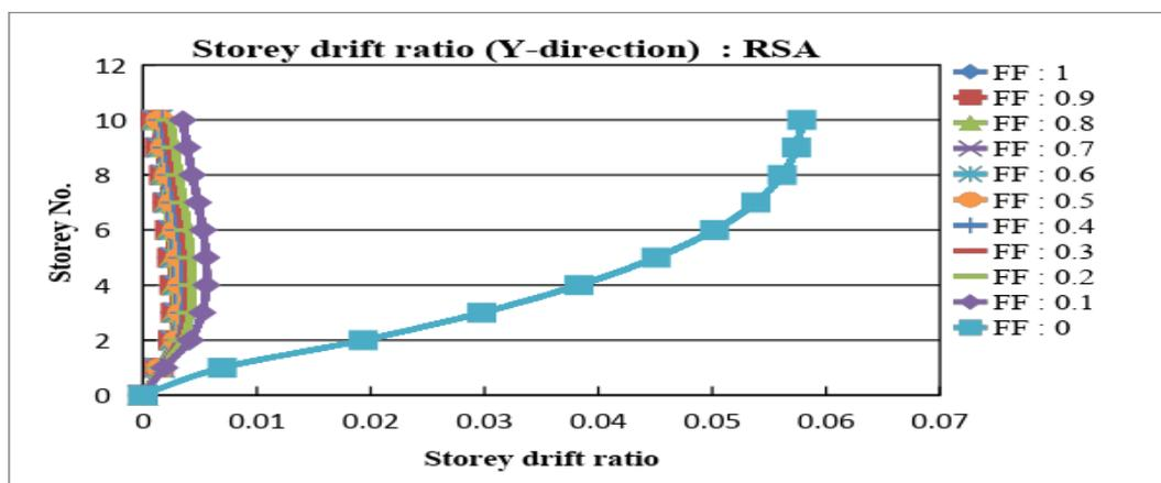
Fig. 9 : Variation of storey drift ratio for all the fixity factors predicted by RSA in Y-direction
