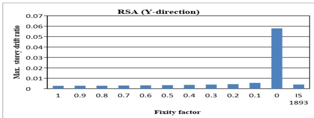
**Fig. 14 : Maximum storey drift ratio predicted by RSA in Y-direction**
