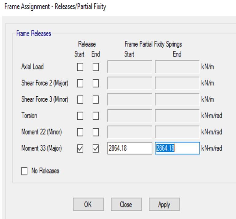
Fig. 5 : Assigning fixity factors in ETABS software
