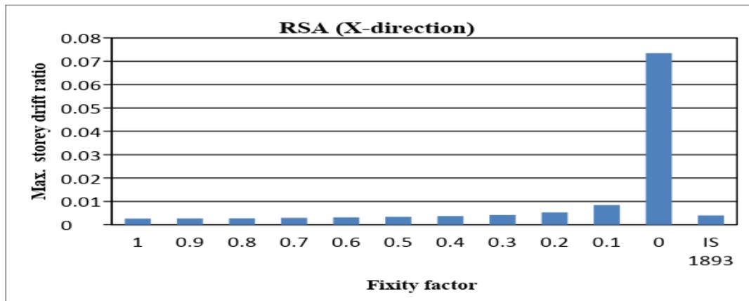
**Fig. 13 : Maximum storey drift ratio predicted by RSA in X-direction**
