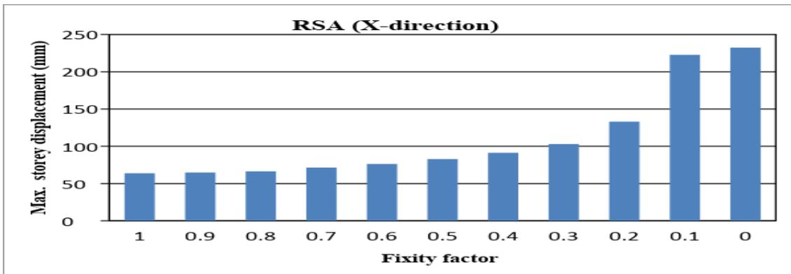
**Fig. 11 : Maximum storey displacement predicted by RSA in X-direction**
