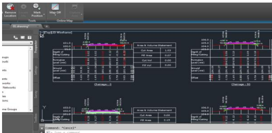
Figure 7 - Cross sections of the road alignment
